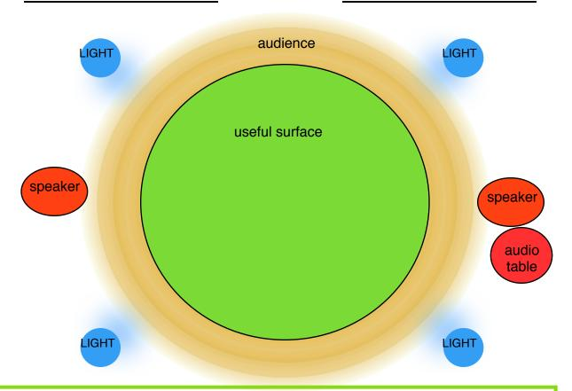
The ideal useful **surface** is 8m in diameter for 7m in height. It must be hard, smooth, stable, level and adherent. (For example, where you can go on roller skates). The LINOLIUM is ideal.
